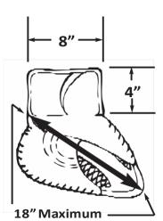
The distance from the heel of the glove along the pocket and following the contour of the inside of the trap of the glove to the top of the "T" trap must not exceed eighteen inches (18"). The heel is considered to be the point at which the straight vertical line from the cuff meets the glove (see diagram at right).
